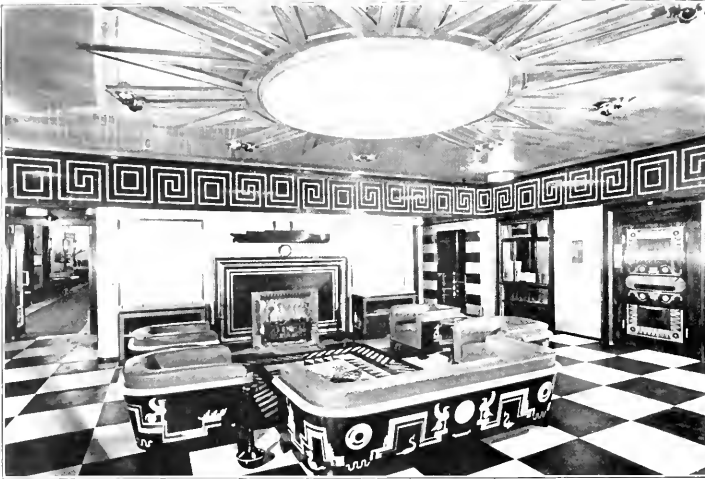
Above, an interesting application of long trough lighting units, which, combined with color changes, produce artistic lighting effects in the Night Club of the Steamship Leviathan.
